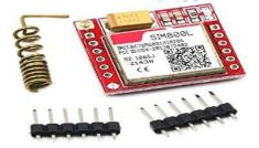
A specialized piece of hardware known as a GSM (Global System for Mobile Communications) module makes use of GSM technology to facilitate communication via cellular networks. An apparatus that facilitates communication between electronic devices over the GSM network is called a
