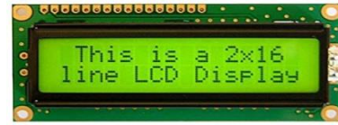
Fig. 5. 16x2 LCD Display with inbuilt driver
